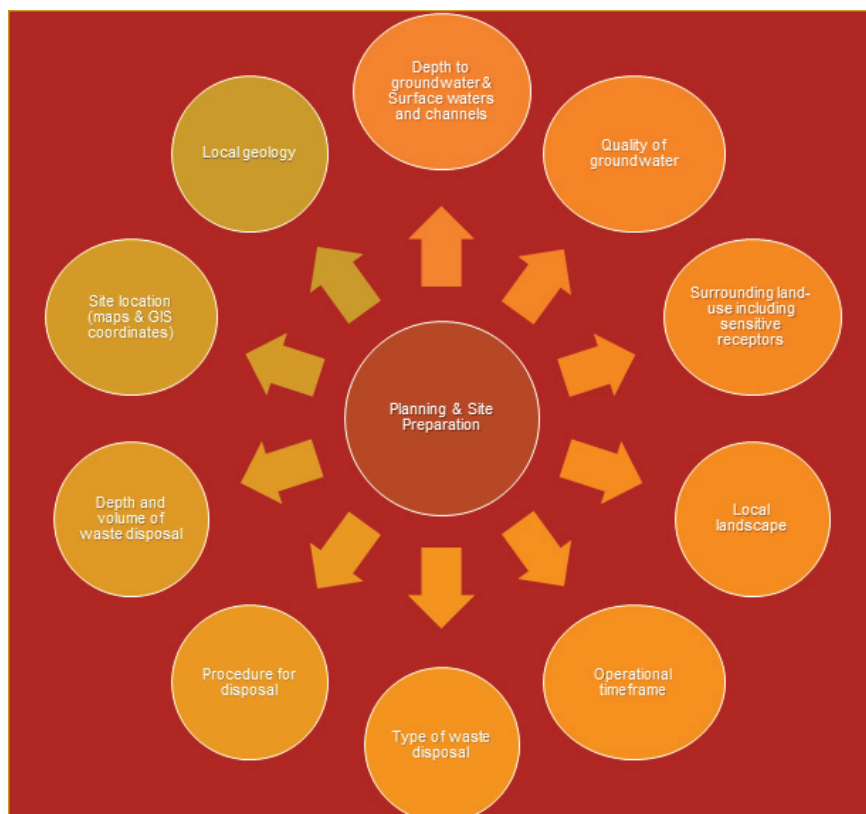
Figure 2: Components to be considered in planning and site preparation
