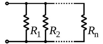
$$1/R_{eq} = 1/R_1 + 1/R_2 + \dots + 1/R_n$$
